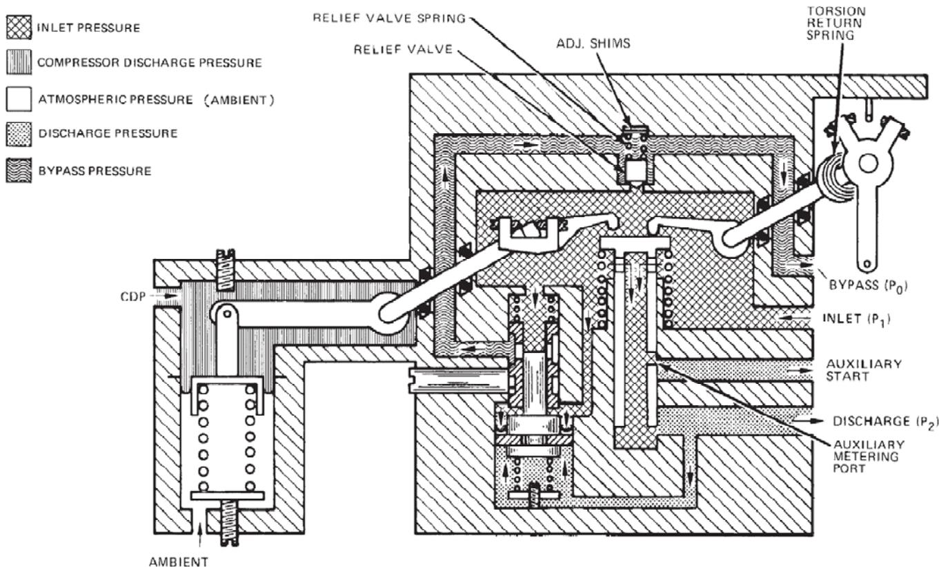
Figure 3. 1907 Liquid Fuel Valve/Limiter with Auxiliary Features
